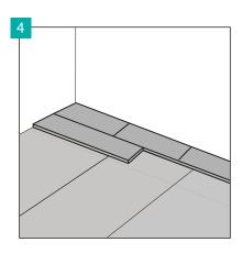
The panels must be laid perpendicularly to the direction of unfolding of the installation mat. Before the panels are glued to the installation mat, spread the panels on the surface and check their location. The panels should be laid in such a manner as to overlap a given ribbon of the installation mat
