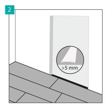
The joints of the neighbouring floor covers must be finished with decorative profiles, leaving expansion joints indicated by the manufacturer.
