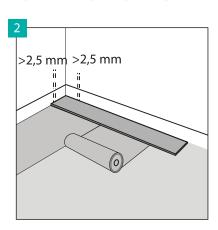
Leave 2.5 mm of perimeter space at the walls to allow the floor expansion. The maximum surface which can be laid without additional expansion joints is 100 m². Above this surface, apply an additional expansion joint and enlarge all the expansion joints up to 5 mm. The maximum length of the floor surface in one direction, which can be laid without additional expansion joints is 10 m. Above this length, apply an additional expansion joint and enlarge all the expansion joints up to 5 mm.
