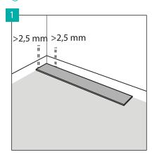
Leave 2.5 mm of perimeter space at the walls to allow the floor expansion. The maximum surface which can be laid without additional expansion joints is 200 m². Above this surface, apply an additional expansion joint and enlarge all the expansion joints up to 5 mm. The maximum length of the floor surface in one direction, which can be laid without additional expansion joints is 20 m. Above this length, apply an additional expansion joint and enlarge all the expansion joints up to 5 mm.
