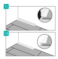
Expansion joints along the walls must be covered with a decorative strip, assembling it by means of an adhesive or special clips. It is recommended to use the Arbiton strips dedicated to a given panel, which guarantee the excellent colour match and the coat resistant to scratching.
