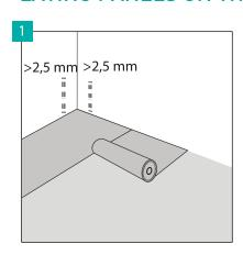
Lay Arbiton Multiprotec LVT Fastlay HD or Ewifoam Vinlay Rapid HD in a direction perpendicular to the direction in which panels are laid, maintaining the 2.5 mm wall expansion joint. The neighbouring underlay ribbons must be fitted to each other, without leaving any unnecessary space.
