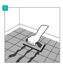
In the case of installation on the substrate covered with ceramic tiles, fill the tile joints with a durable compound for the filling of points, e.g. resin grout is recommended. While using the mat with the Arbiton Multiprotec LVT Fastlay or Ewifoam Vinlay Rapid HD adhesive layers, it is not necessary to fill the tile joints with a point thickness up to 3 mm and depth of 1.5 mm.
