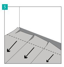
Remove a part of the protective film and glue the panels to the uncovered adhesive, laying them tightly next to each other, without leaving any gaps. The adhesive on the protective mat may be uncovered for no longer than 30 minutes, and at this time, panels must be glued to it.
