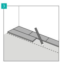
Determine the reference line to cover a part of the substrate with an adhesive, so as to glue the panels.
