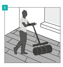
Not later than 30 minutes after gluing the panels, use a heavy roller in order to press the glued panels to the substrate accurately and evenly.
