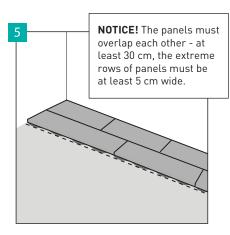
Glue the panels to the substrate by laying them tightly to one another, without leaving any gaps. The laying of the first line of panels perfectly straight will affect the good visual effect of the whole room.
