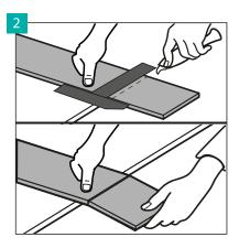
For additional cutting of floor panels, use a sharp knife, cut the top layer, then break the panel by leaning it on the edge.
